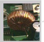
Inductors are used in many applications, from filters to florescent lighting and ignition units.
