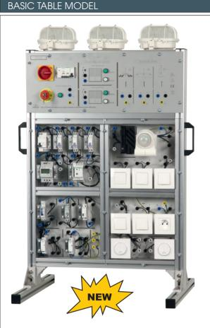
This compact model can be placed on a table; it brings together the same components as the TAG-2 reference model on a frame with rollers (the convector is found on the back). It therefore satisfies the same teaching goals, and can perform all the practical works.
